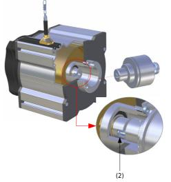
By tightening the radial screw the encoder will be clamped and secured from twisting. Please use a hexagon screwdriver, size 3.
