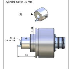
Please mount the encoder into the easy-clamp-flange. The cylinder bolt must slip into the spring (2).
